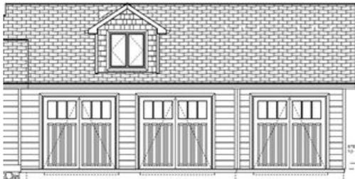
I took it a step further, though, so as to not just point out an issue, but more importantly how to solve the issue! I modeled the garage roof using conventional stick framing and elevated the ceiling joists/collar ties to give him the necessary headroom. I modified the elevation shown, using a dormer over the double bay section, by making the dormer wider and centered over center bay, which is where he wanted to work on the vehicles/have taller lift.
